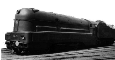
SNCF 2-3-2 P-1 and DR 19.10001 as running locomotives The only two individual-axle-drive prototypes completed
