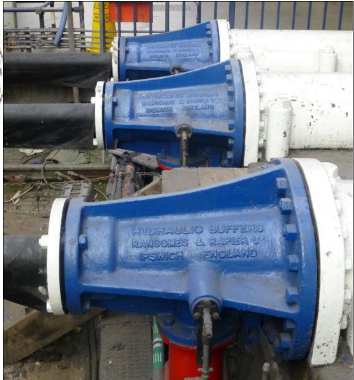
Hydraulic buffers at London Waterloo made by Ransomes & Rapier, Ipswich, probably some ninety yeas ago. Photo 4 November 2024 John Billard
