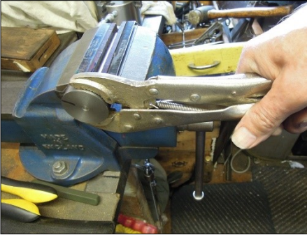
Screwing the piston on to the rod. Not for the faint hearted!
