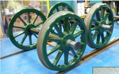
Left New matched wheels as part of the 2006 restoration
