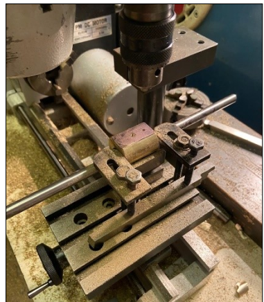
Bottom right Milling and drilling the cylinder block on the milling table, which is attached to the lathe cross-slide
