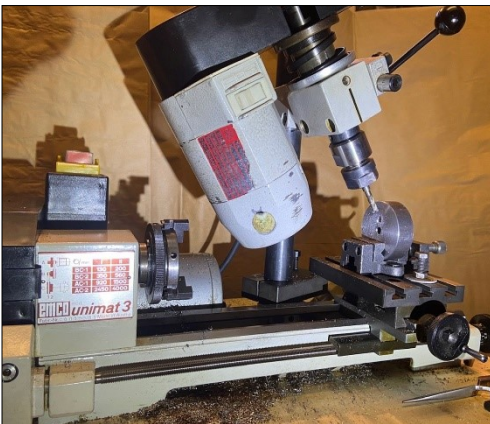
Top right Drilling the engine frame with the faceplate mounted on the tailstock
