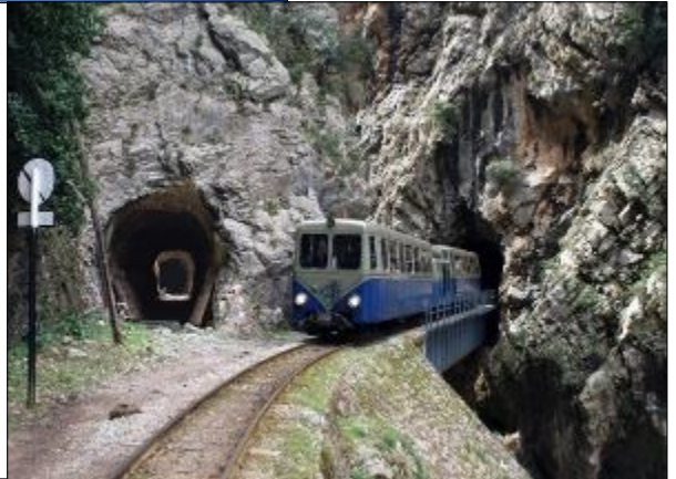
A 1967 Decauville set at a location called the Portes near the top of the Gorge. Old alignment to the left. Note the “sandwiched” diesel-electric generator car.
