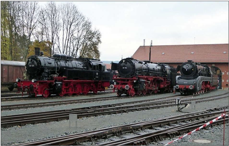
Locos outside the museum at Neuenmarkt. 2-8-2T 93-526, high speed 3-cyl Pacifics 01-164 and 10 001.
