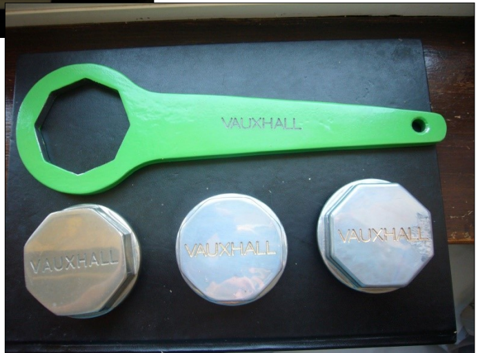
Right , a special spanner made from 10 mm steel using the plasma cutter + CNC
