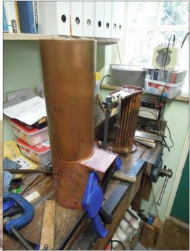
Not quite so much to report this month However I have been consulting with the RSME boiler inspectors being unsure about the crucial joint between the boiler barrel and the firebox This led me to talk to Western Steam who supplied my boiler kit. It turns out that a jointing ring was omitted and I hope that this is now on its way. We discussed whether it was necessary to flange the throat plate against the barrel and Western Steam said no. But I knew that our inspectors preferred it that way.
