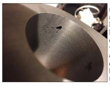
steel bar with centres drilled on either end and a square cross hole to take a tool bit, held by grub screws. Some might ask how it is possible to bore to a size without any fine adjustment. My technique was to carefully measure the protrusion of the toolbit from the boring bar, using a digital caliper. This technique resulted in both cylinder bores to within a thou of the target dimension.
