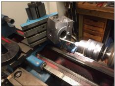
inder bore. The same error occurred on both cylinders and was presumably caused by the lathe cross slide surface not being parallel to the lathe axis. I suppose this is not a surprise on an old lathe, as the forces on the saddle are nearly always at one end only, which will result in uneven wear. The issue with the cylinder blocks was easily rectified by using the mill to fly cut away a few thou to true it up.
