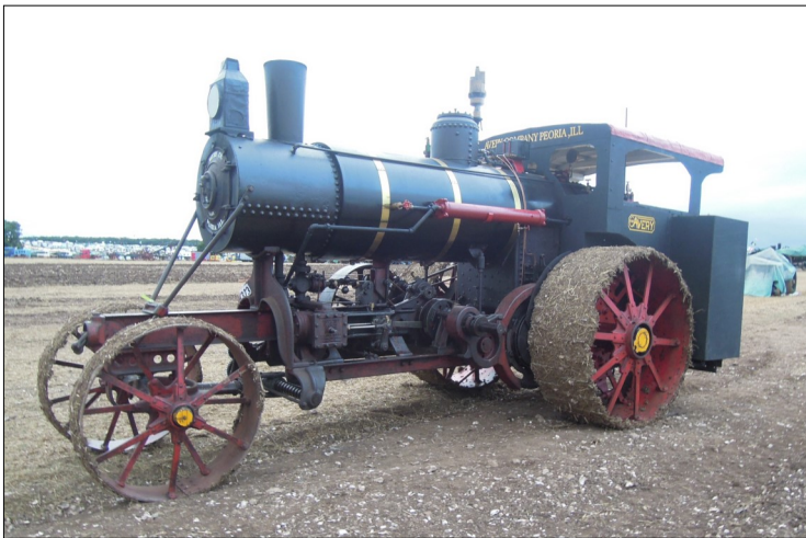
A USA built Avery agricultural tractor used for direct haulage ploughing.
