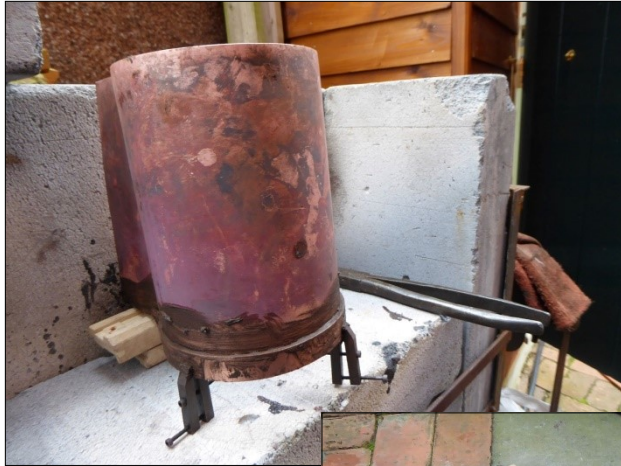
Left The reinforcing ring fluxed up and ready to go.
