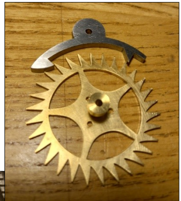
Left The start of cutting the pallets out of 1/8" gauge plate.
