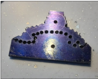
Left The start of cutting the pallets out of 1/8" gauge plate.
