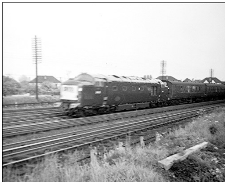
Prototype diesel DP2 at Northwick Park. A Class 50 in a Deltic body shell.
