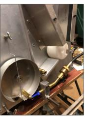
the duration and temperature of annealing can be controlled *(Photo left over-leaf)* shows the effect of different annealing durations. The cartridge at the top is correctly annealed). Some components of the device are interchangeable to accommodate cartridge cases of different sizes.
