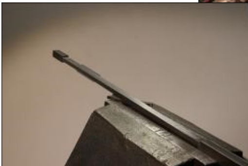
Left Filing the sides of the reach rod. Notice the subtle bowing.
