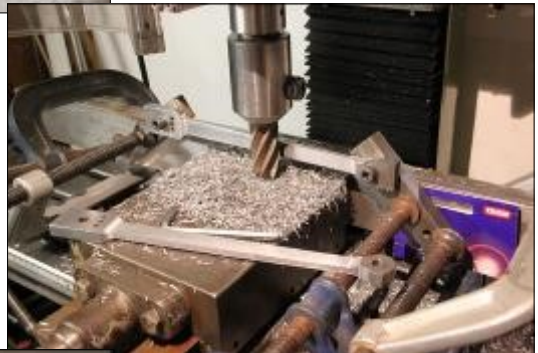
Right Milling the main rods - a lovely set up that can be used for all sizes.
