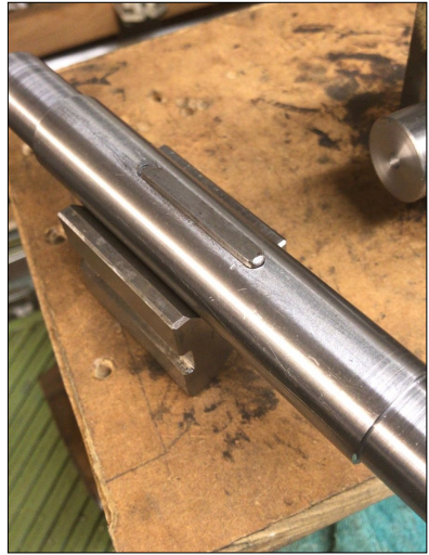
Above left machining the keyway in the new axle Right with the keys in place Left Assembled with the pump eccentrics.
