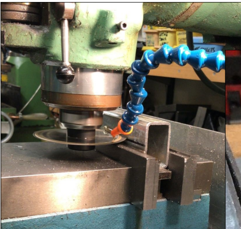
Slitting box section steel to form the coupling brackets
