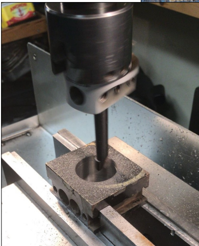
The axle box being bored and complete.
