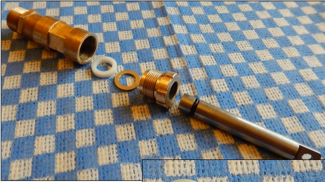
The axle pump ram fitted with the new "O" ring and the new PTFE bearing and brass backing washer.
