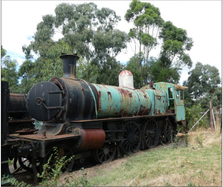
D3 646 4-6-0 awaiting repair at Maldon
