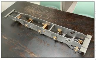
So far, I have made a start good on the frames These were supplied as sheets of 1/8" steel flats, to which I applied engineer's blue and then spent a satisfying evening of marking-out on the kitchen table. These were then sawn and filed in "the old school way", along with some
