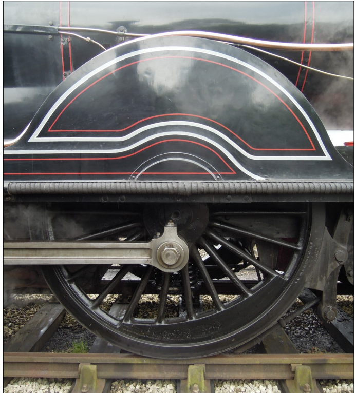
Driving wheel of LSWR T9 4-4-0 at Quainton on 1 May 2017. Photo John Billard
