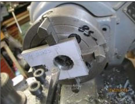
Boring a very accurate hole, converted into metric!
