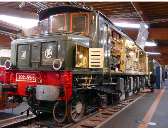
1500 V DC locomotive with wheel configuration 2-D-2.
