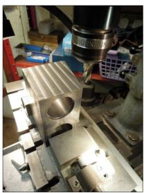
Having replaced the defective casting all outside surfaces were machined to size. Then Nigel Penford very kindly agreed to allow me to use his Bridgeport milling machine to complete the bores. **See the top photo.** This was quite a long job.
