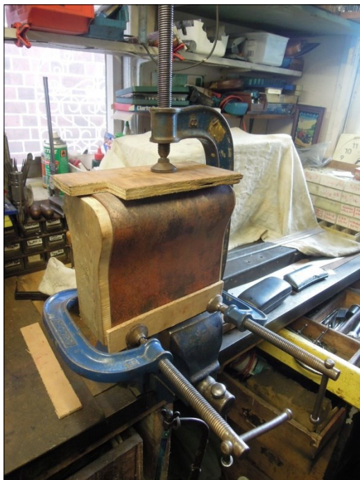
Top Left The back head partly drilled and the firehole ring is tried in place.
