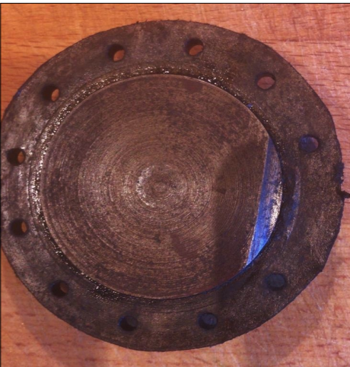
Below Cylinder end cover with impact mark
