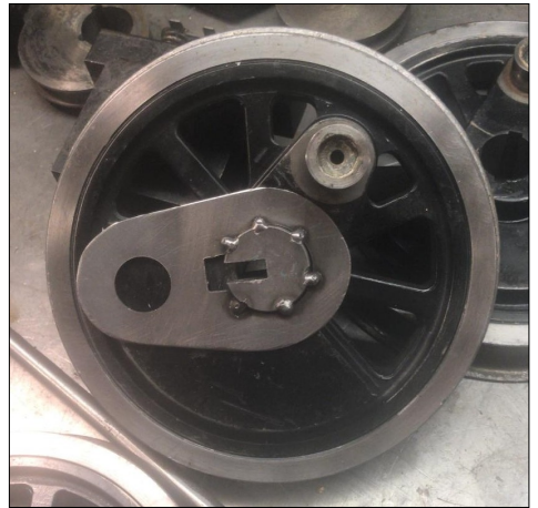
Left Stepped key being machined - not easy to hold!
