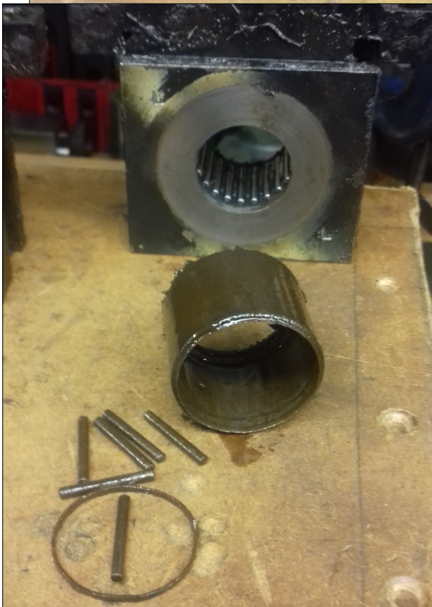
Above The axle pump eccentrics. Very dirty but otherwise quite serviceable.
