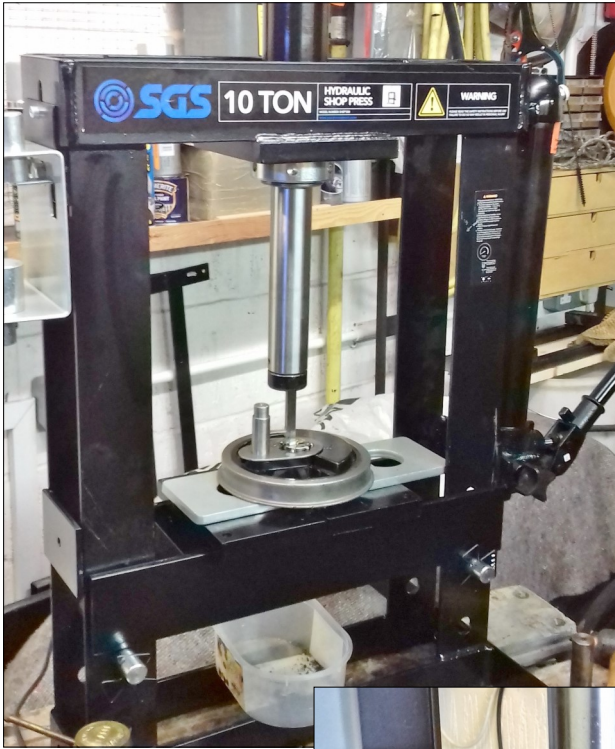
Broaching the key way with the 10 ton press.
